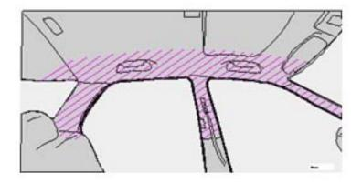
• The VIC system is a supplement to the Side Impact Protection System. It is not designed to deploy during collisions from the front or rear of the car or in rollover situations.
